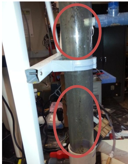
Figure 4.9: Colloidal material attached to feed tank walls
