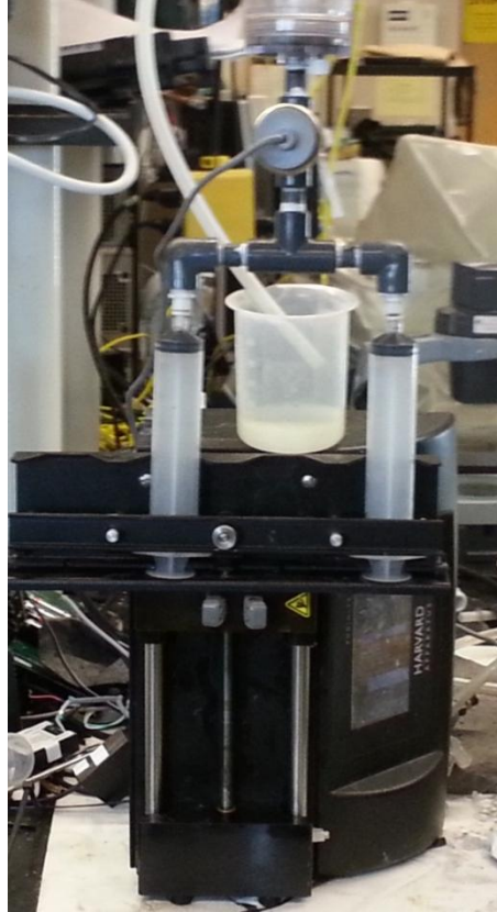
Figure 6.1: Syringe pump setup for the Modified Fouling Index testing
